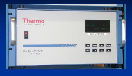
The hourly SO<sub>2</sub> was measured by pulsed fluorescence (model 43-C SO<sub>2</sub> monitor, Thermo Environmental Instruments, formerly Thermo Electron Corporation (TECO), Cheswick, PA, USA). These instruments were set up to auto calibrate once every 24 hours by EPA approved methods (span and zero gas and flow stream switching).
