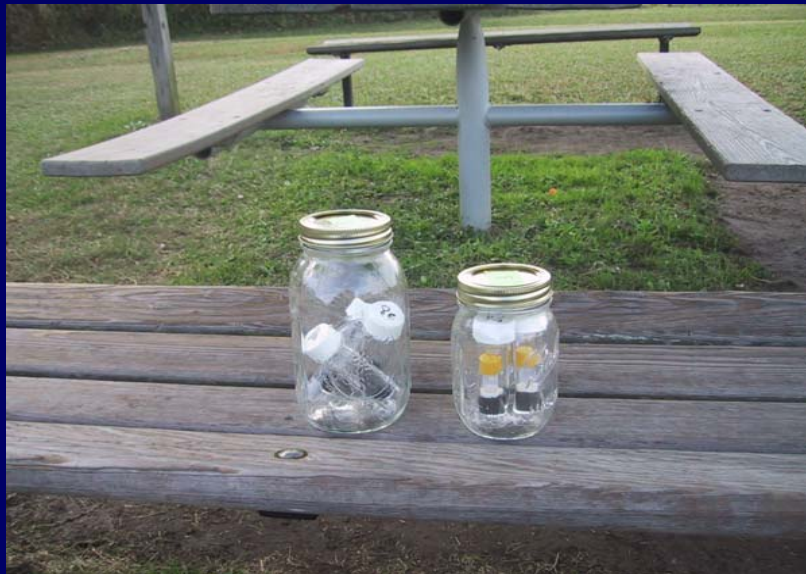
Picture of \text{NH}_3 diffusion tubes in collection jars
