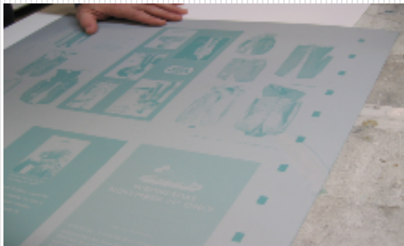
Plate with image to be printed
