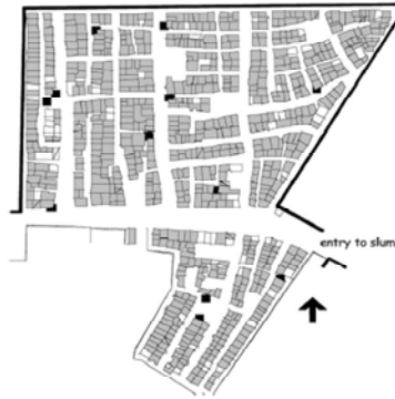
Fig. 8. Gandhinagar, Yerawada. The grey-shaded houses have their own water. The black squares are common water points. Even the houses with the water points exactly at their door step have their own connections.
