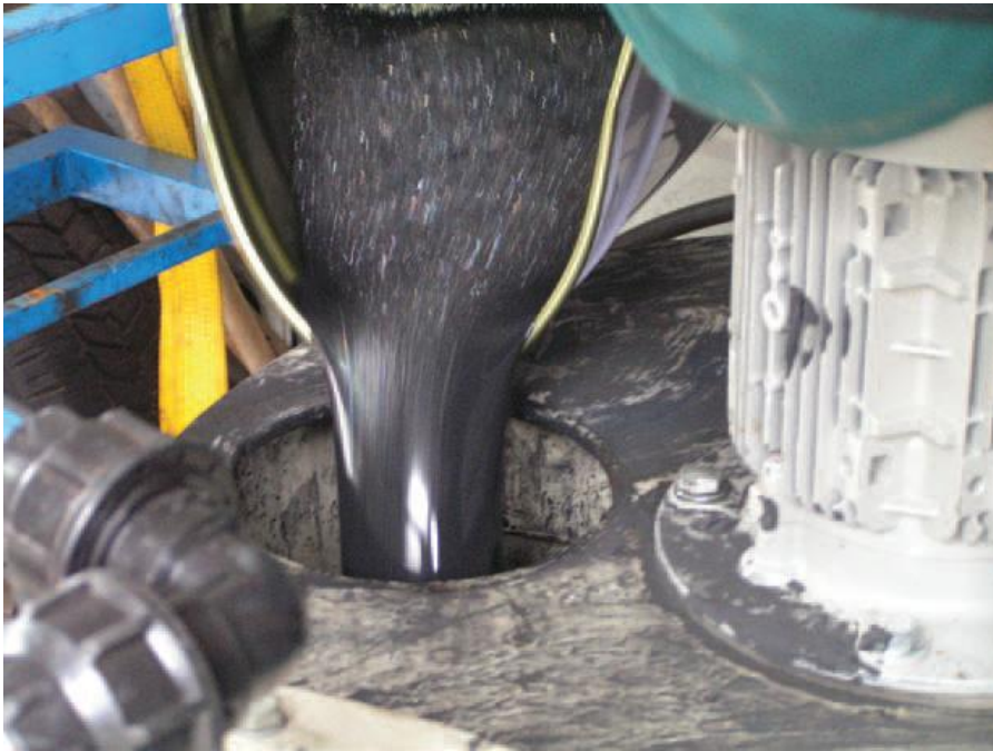
pouring of nZVI slurry into a water well
